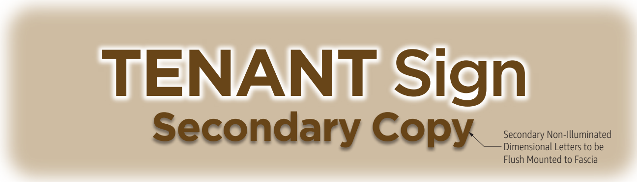
Halo Illum. Letters with Non-Illum. Dimensional Secondary Copy (at Tenant's Discretion)
